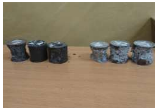
Fig. 2. On the left is a view of the molded samples. On the right is a view of the samples following their compressive strength test after 28 days
