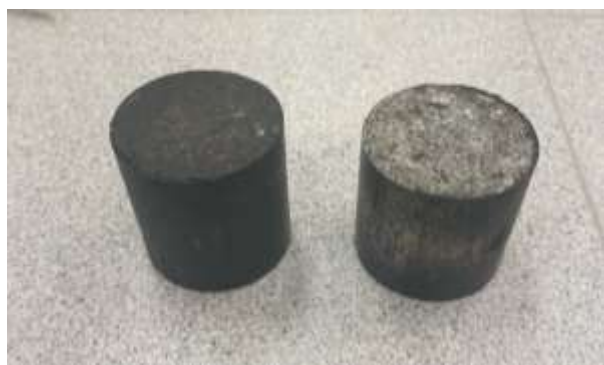
Fig. 2. On the left is a view of the molded samples. On the right is a view of the samples following their compressive strength test after 28 days
