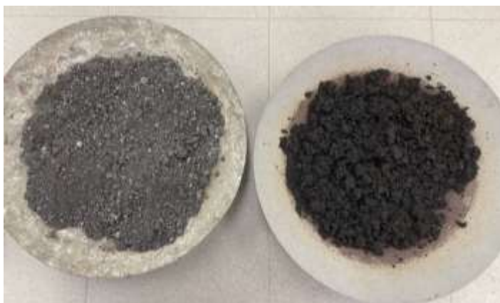
Fig. 1. On the left is a view of humusized soil treated with 5 % lime, on the right is a view of humusized soil not treated with limestone
