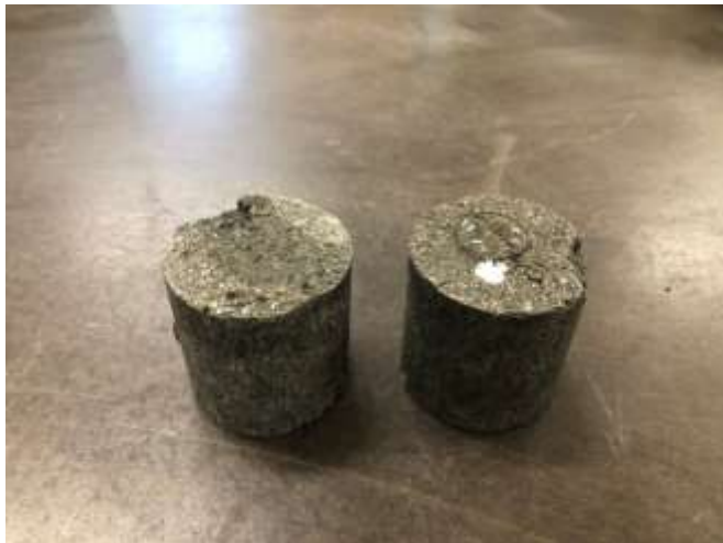
Fig. Type of the samples after water penetration. On the left is a sample with no modifier, on the right is a sample with a MADOR modifier
